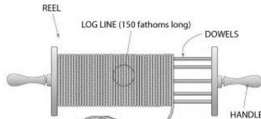
Figure 6. Parts of the Reel
